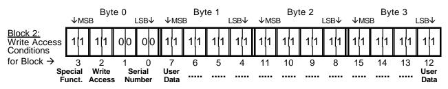
The ones in the 16 pairs of bits have to be cleared together if the corresponding block is wanted to be write protected forever  $(1|1 \rightarrow \text{write access enabled}, 0|0 \rightarrow \text{write access disabled})$ . Writing of bit pairs 1|0 or 0|1 to block 2 is not allowed!
