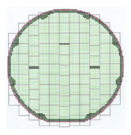
The three black lines show the position of the PCM structures on the 6 inch wafer!
